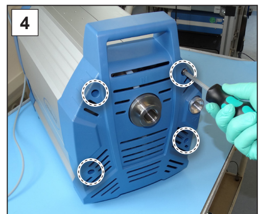
4. Wind in the 4 screws of the front housing section; hex key size 4.
