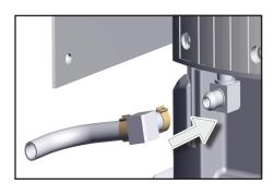
➡ Slip the elbow fitting of the connection hose (included in shipment) and a hose clip (also included) onto the elbow fitting of the pump.
