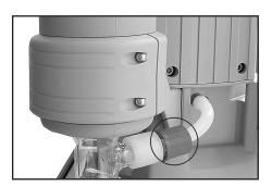
Loosen the union nut at the inlet of the exhaust waste vapor condenser.
