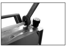
→ Use an open-ended wrench (width 17 mm) to loosen the union nut at the hose connection next to the gas ballast.
