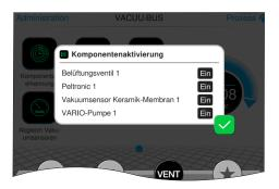
Using **component activation**, a connected Peltronic condenser can be individually activated or deactivated, i.e., the Peltronic condenser can remain connected but is switched on or off at the controller as required for the ongoing process.
