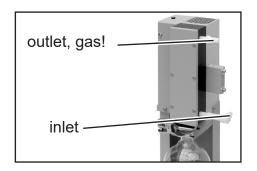
The **exhaust waste vapor condenser Peltronic** enables an efficient condensation of the pumped vapors at the outlet. The condenser's temperature is automatically controlled to +50 °F (+10 °C).
