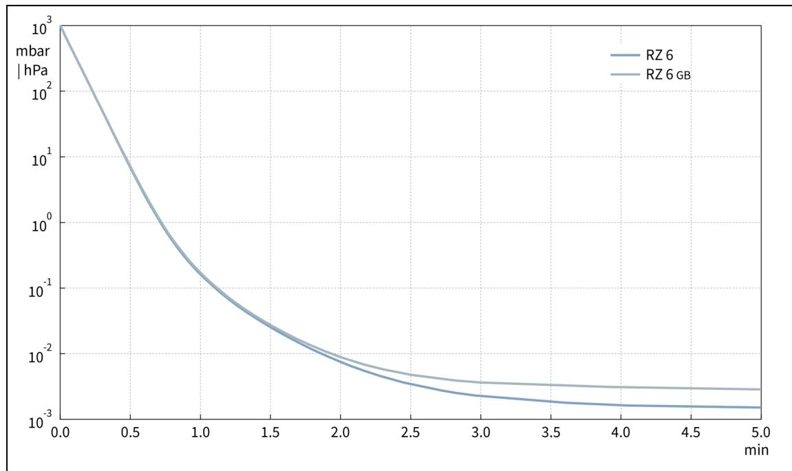
**Gráfico de caudal de aspiración a 60 Hz**
