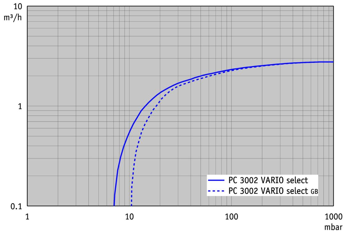
**Courbe de pompage à 50 Hz (réservoir 10 l)**
