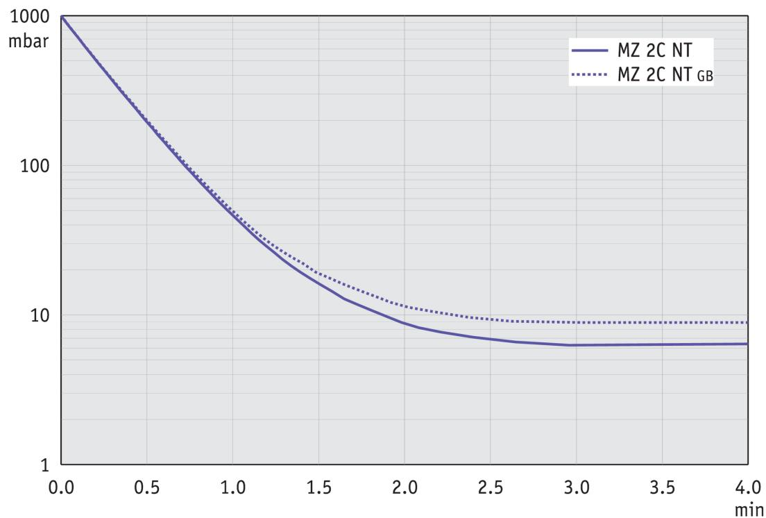
**Courbe de débit à 60 Hz**
