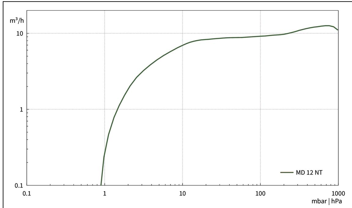
**Courbe de pompage à 50 Hz (réservoir 100l)**
