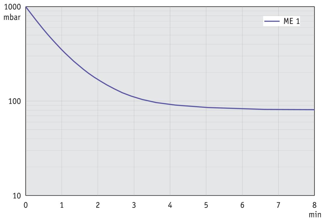
**Courbe de débit à 60 Hz**
