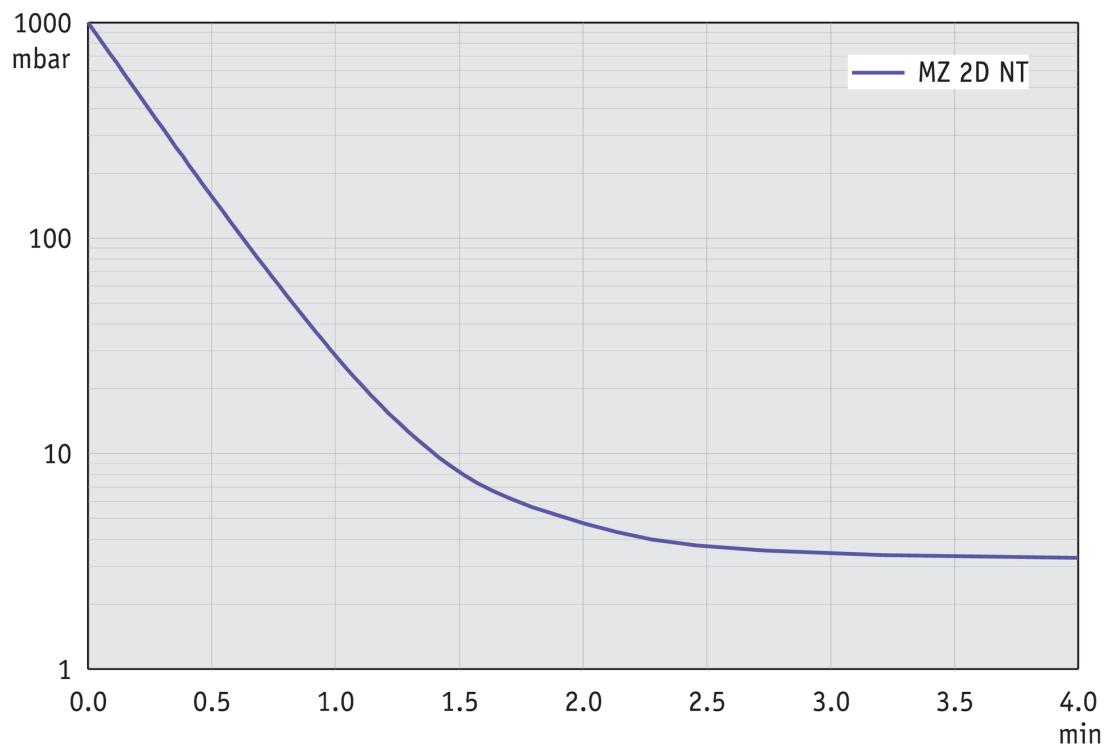
**Courbe de débit à 60 Hz**
