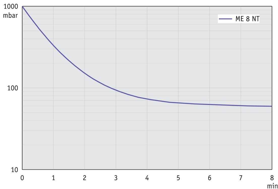
**Courbe de débit à 60 Hz**
