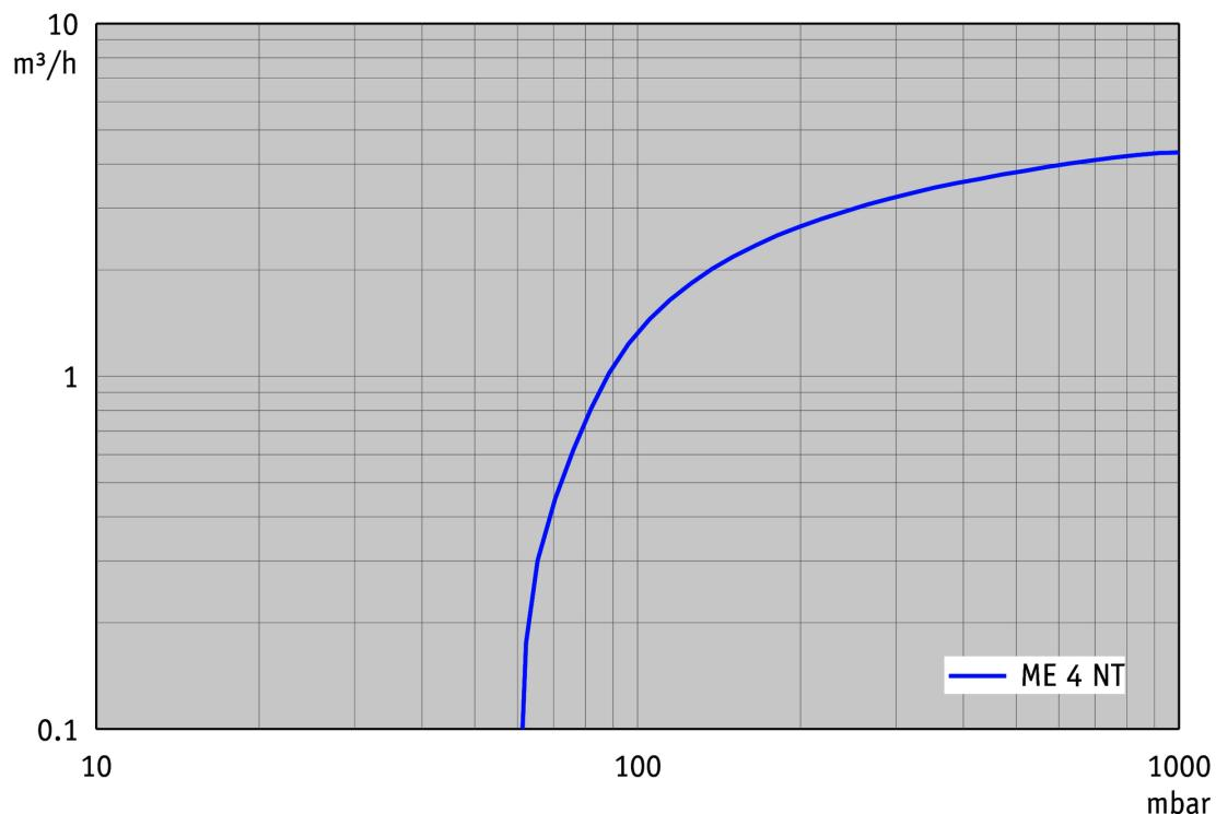
**Courbe de pompage à 60 Hz (réservoir 10 l)**
