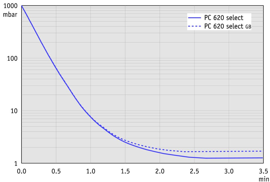
**Saugvermögenskurve bei 60 Hz**
