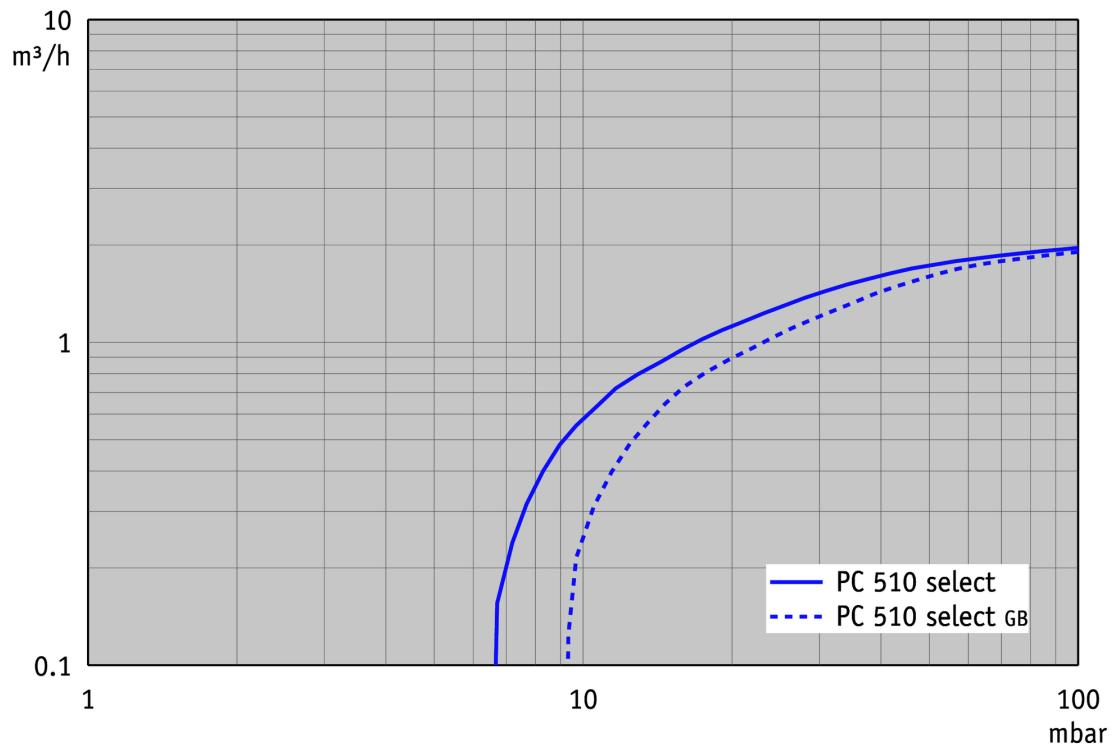
**Abpumpkurve bei 60 Hz (10 l Behälter)**
