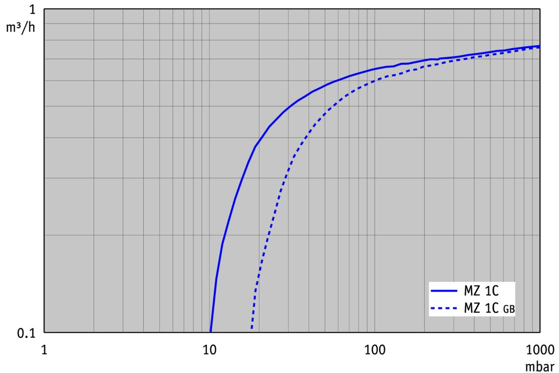
**Abpumpkurve bei 50 Hz (10 l Behälter)**
