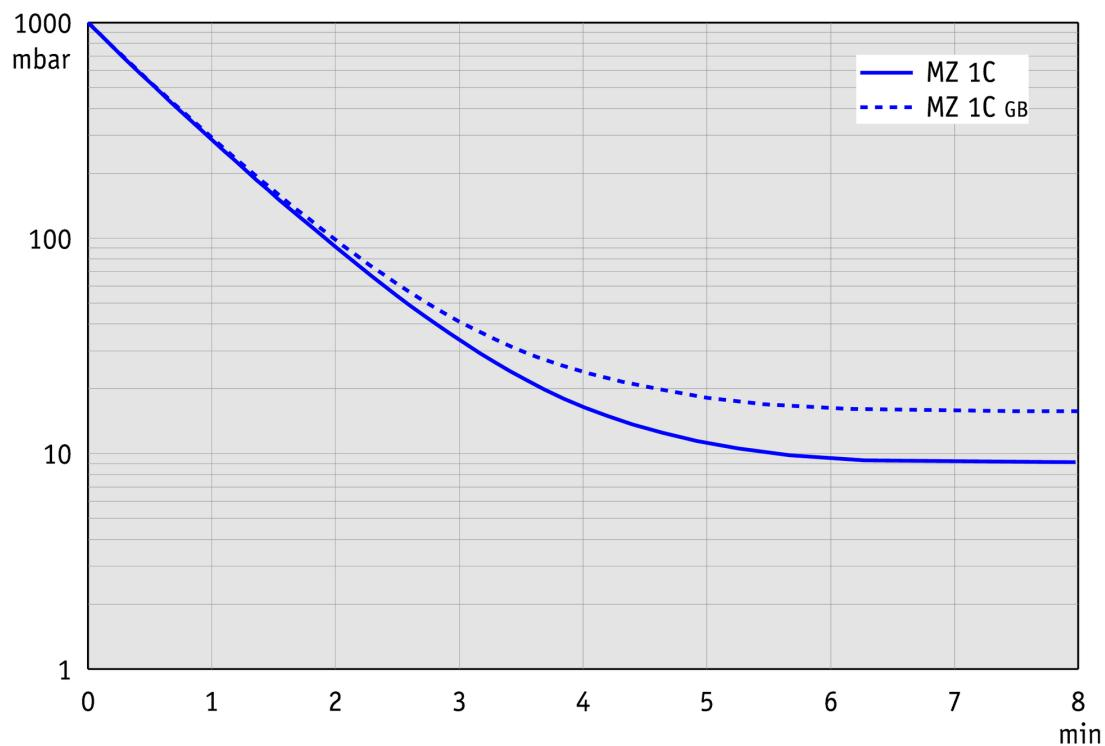
**Saugvermögenskurve bei 60 Hz**
