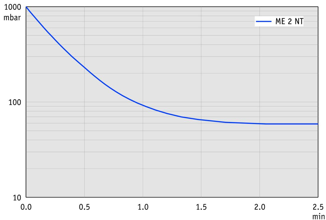
**Saugvermögenskurve bei 60 Hz**
