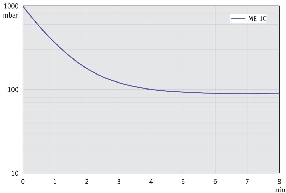
**Saugvermögenskurve bei 60 Hz**
