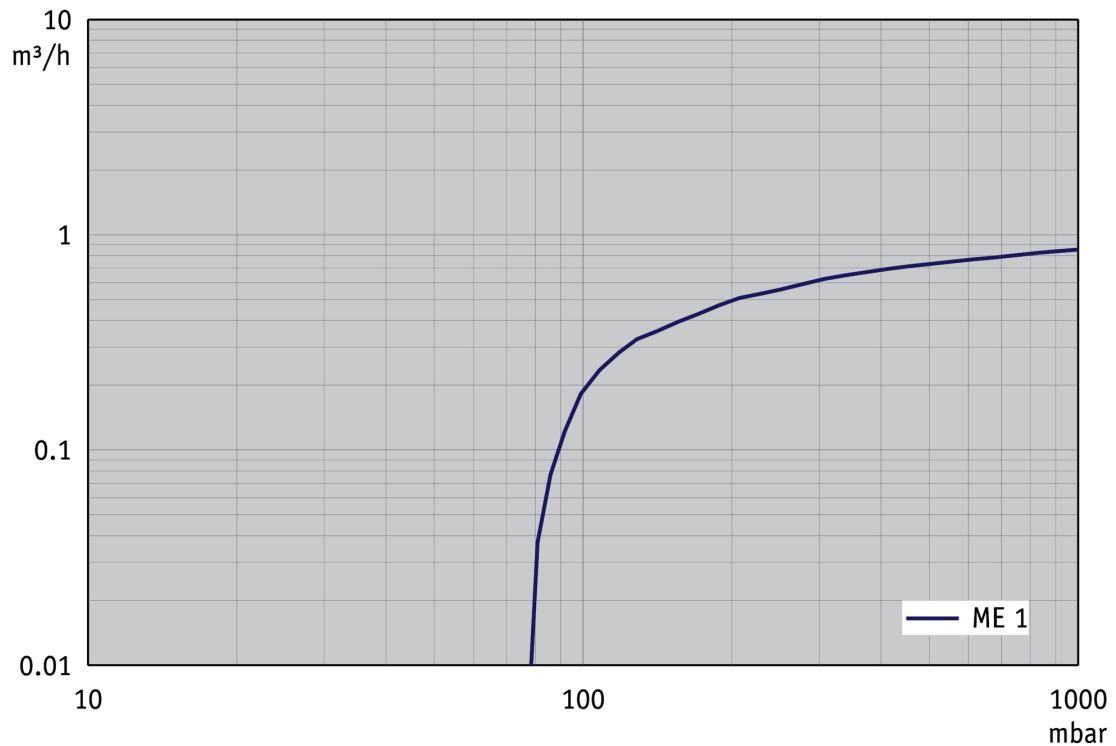
**Abpumpkurve bei 60 Hz (10 l Behälter)**
