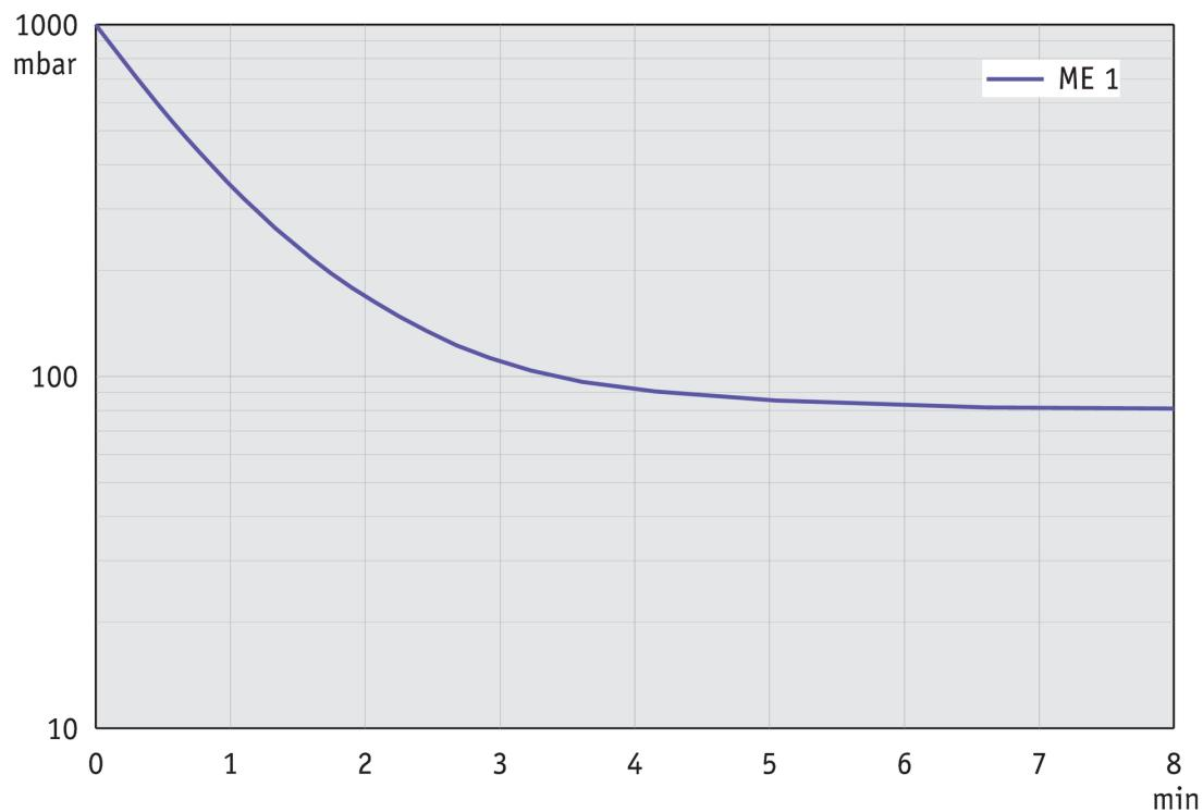
**Saugvermögenskurve bei 60 Hz**
