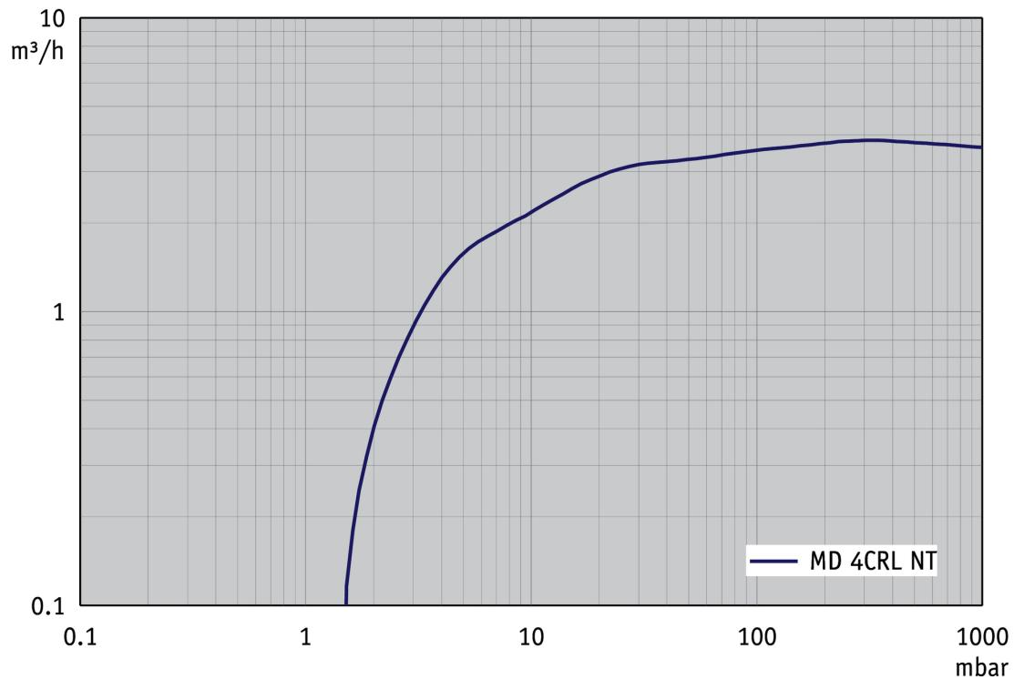
**Abpumpkurve bei 60 Hz (10 l Behälter)**
