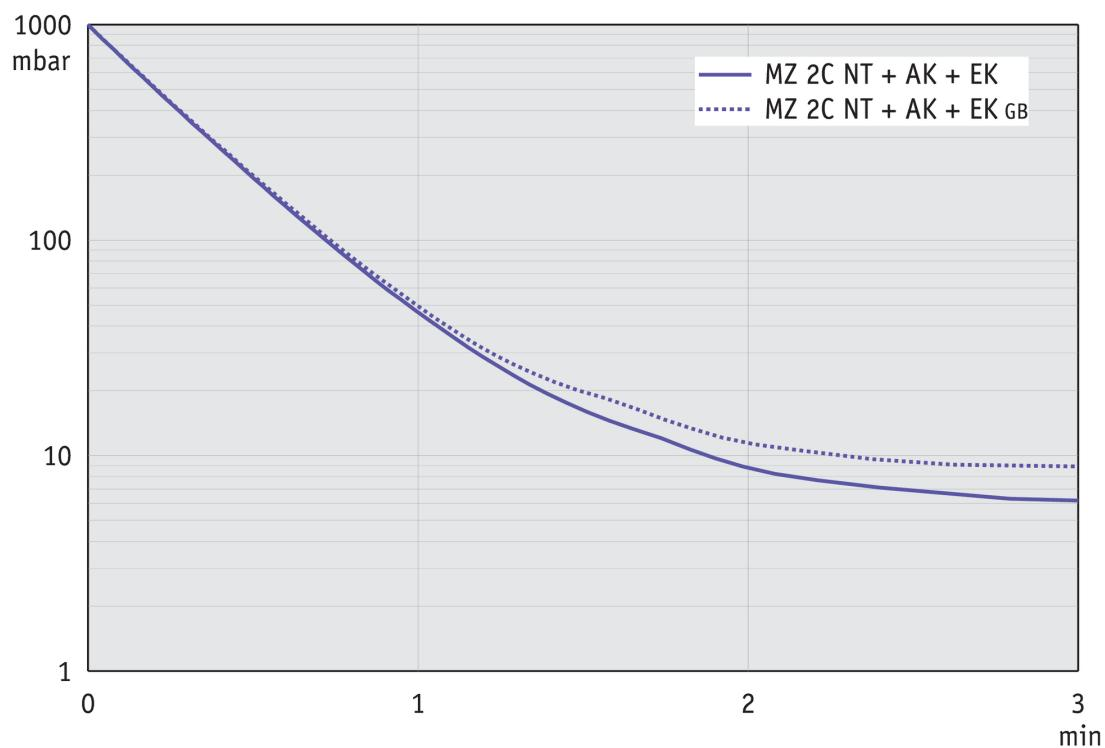
**Saugvermögenskurve bei 60 Hz**
