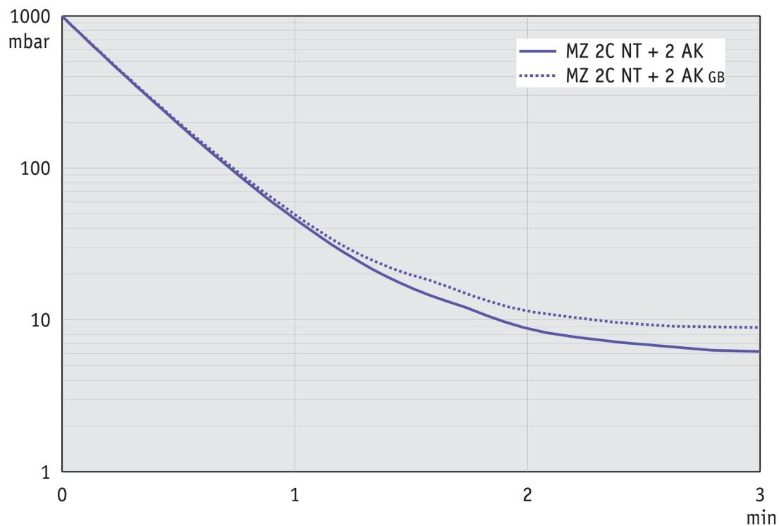
**Saugvermögenskurve bei 60 Hz**
