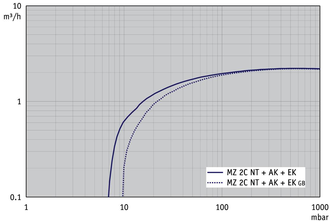
**Abpumpkurve bei 60 Hz (10 l Behälter)**
