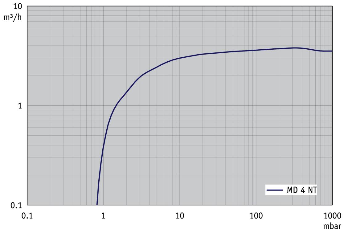
**Abpumpkurve bei 50 Hz (10 l Behälter)**
