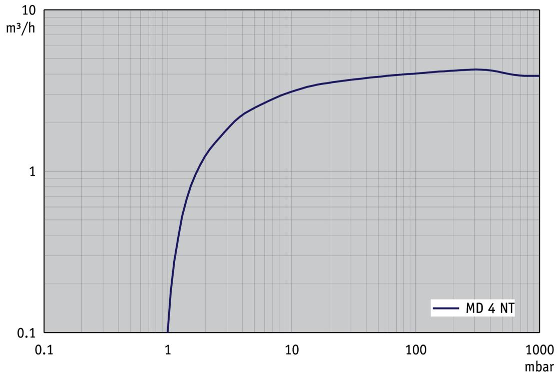
**Abpumpkurve bei 60 Hz (10 l Behälter)**
