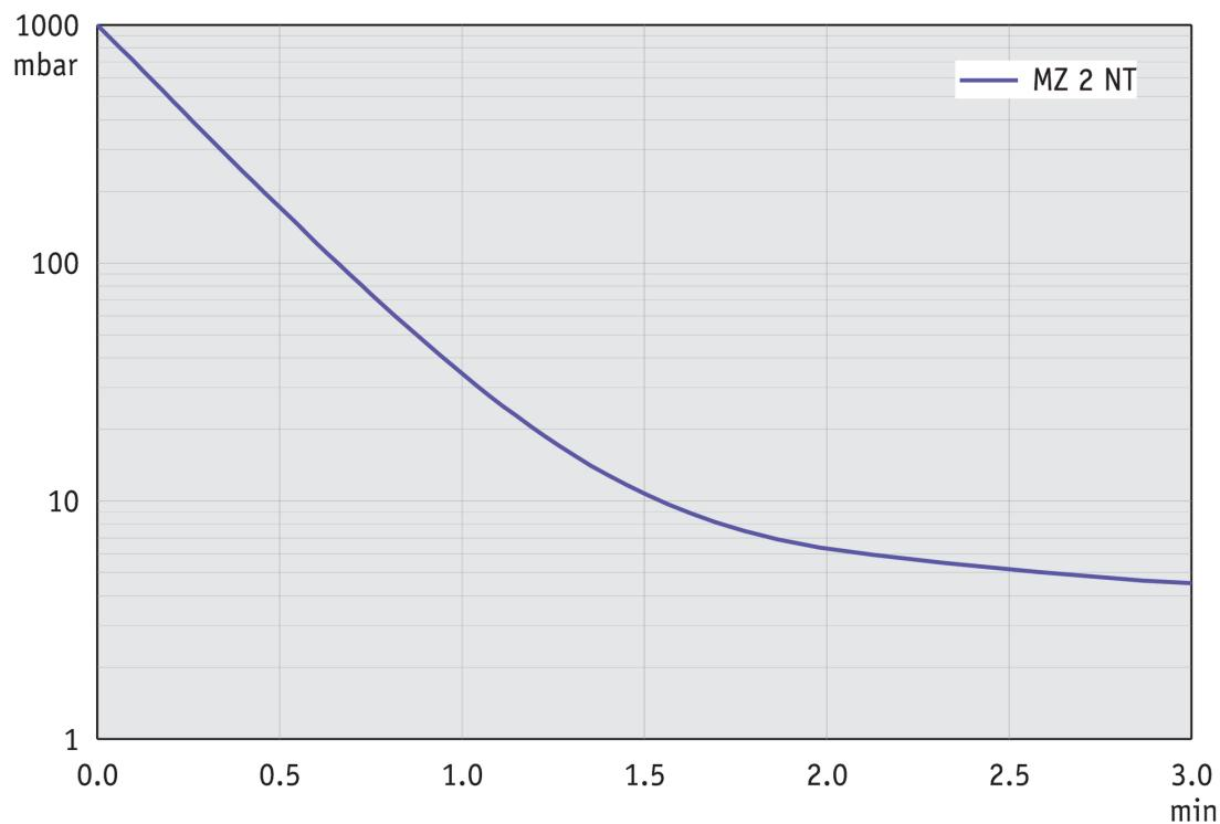
**Saugvermögenskurve bei 60 Hz**
