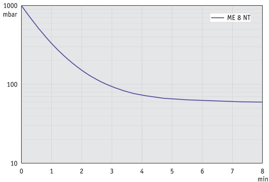
**Saugvermögenskurve bei 60 Hz**
