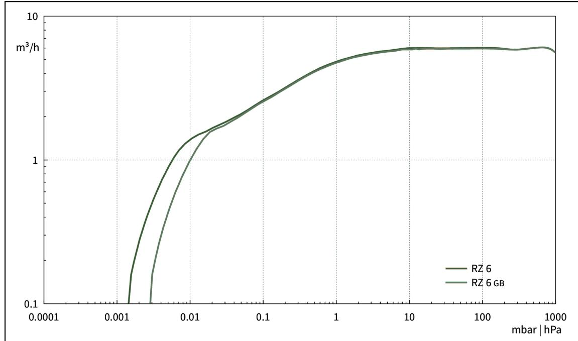
**Abpumpkurve bei 50 Hz (10 l Behälter)**
