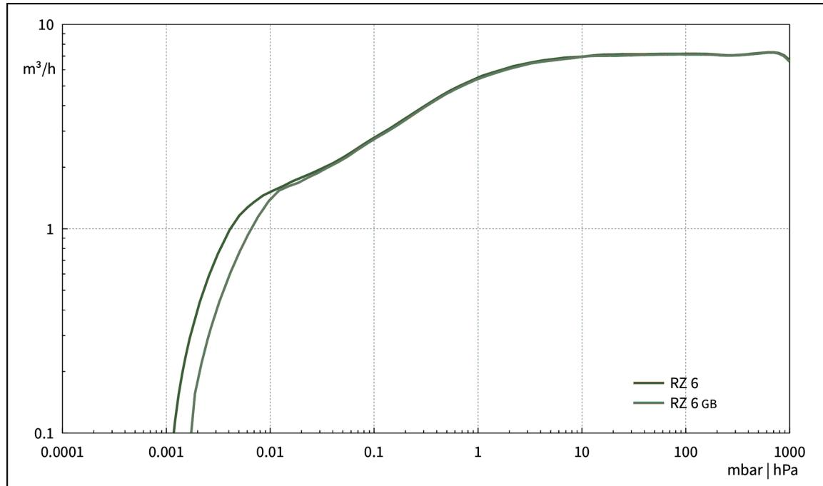
**Abpumpkurve bei 60 Hz (10 l Behälter)**
