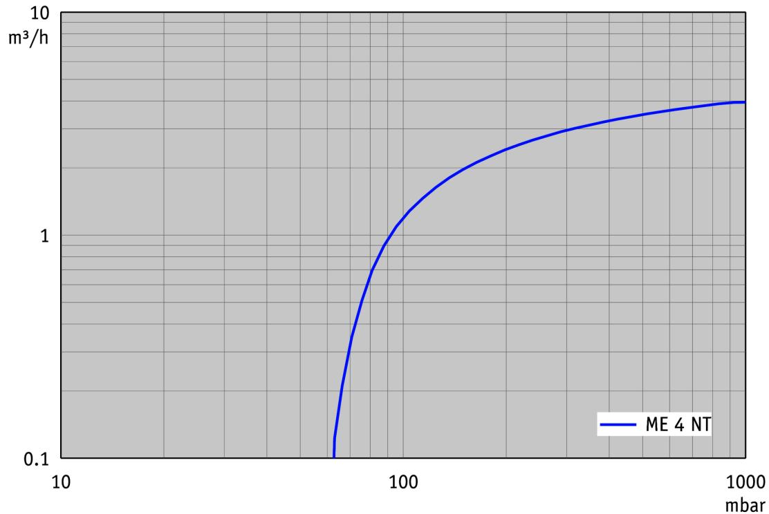
**Abpumpkurve bei 50 Hz (10 l Behälter)**
