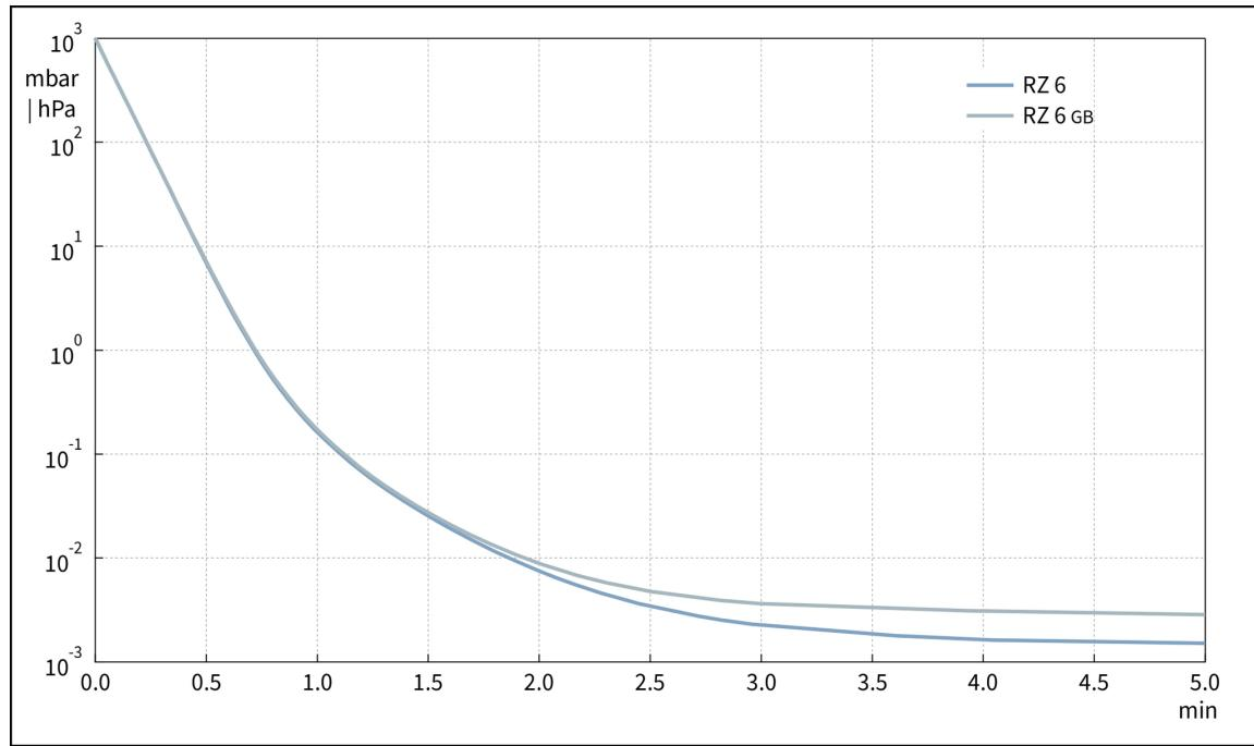
**Saugvermögenskurve bei 60 Hz**
