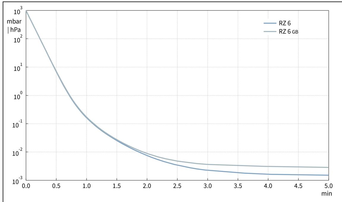
**Saugvermögenskurve bei 60 Hz**
