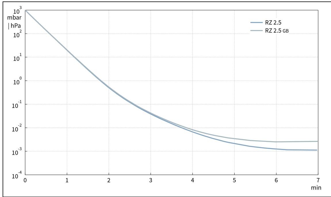
**Saugvermögenskurve bei 60 Hz**
