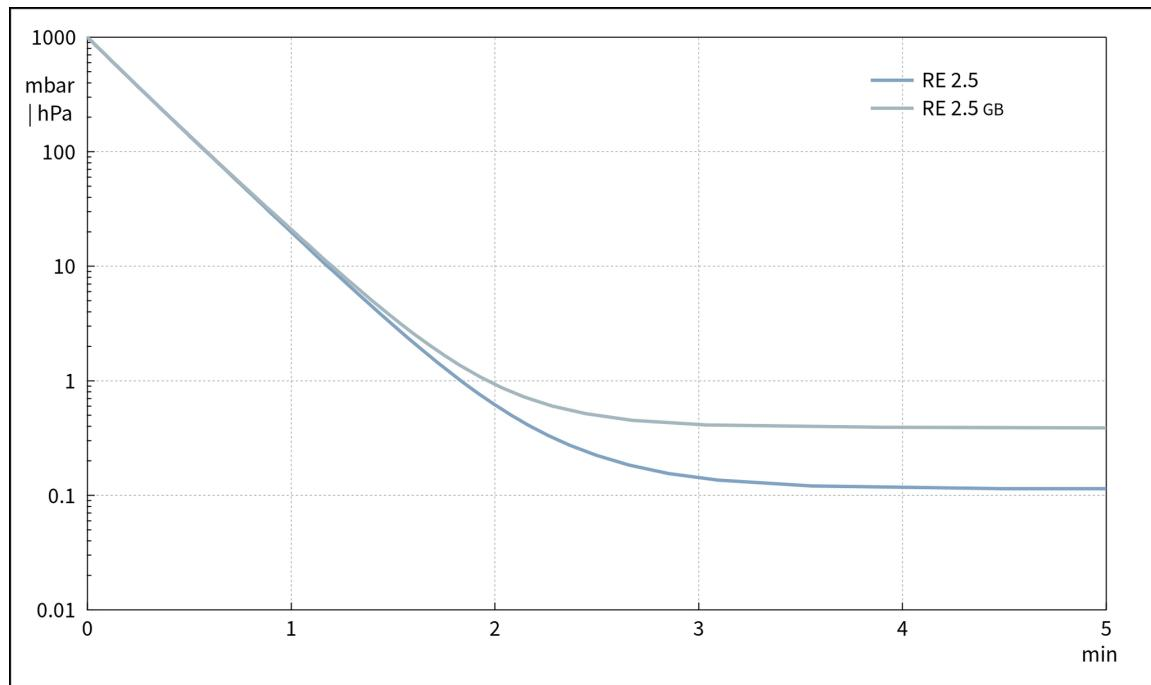
**Saugvermögenskurve bei 60 Hz**
