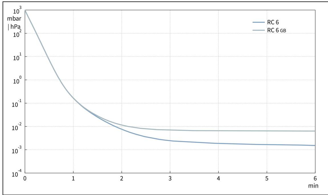
**Saugvermögenskurve bei 60 Hz**
