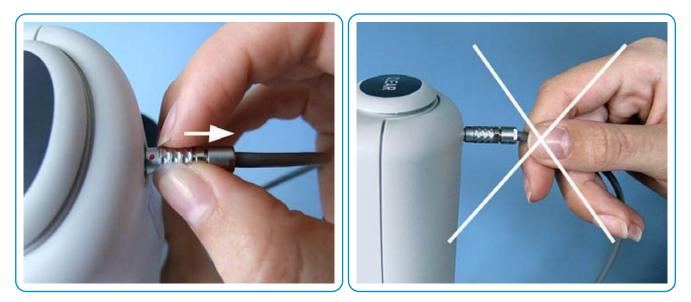
To connect the instrument, plug the cable into the locking socket of the instrument, the red dot facing upwards. To disconnect the instrument draw the sliding sleeve backwards to remove the plug. Never pull on the cable!
