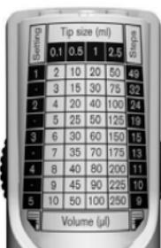
The volume table on back of the instrument is two-sided. To change the table, push the clip up, turn the table around and push the clip back down again.
